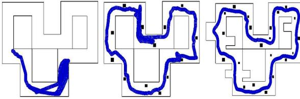
Figure 2: Learning to navigate. Three different environments were introduced to the robot, incrementally increasing the complexity of the world where the robot had to operate. The traces show how the robot gradually adapted to its environment and became able to smoothly navigate through the simulated corridor.
